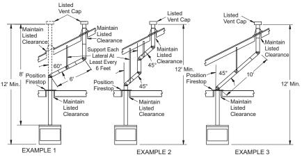
Figure 10 - Typical B-Vent Configuration
